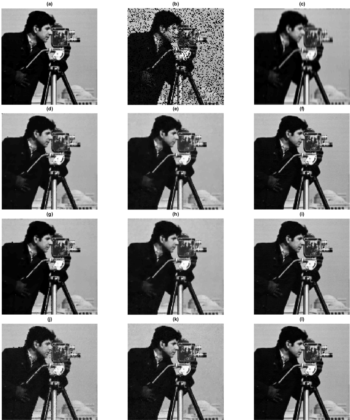
Fig. 1 (a): Original image. (b,c) Observed masked and blurry images. (d, e, f): EWA- \ell_1 estimated images from masked image, compressed sensing measurements, and blurry image. (g, h, i): EWA-FIRM estimated images from masked image, compressed sensing measurements, and blurry image. (j, k, l): EWA-SCAD estimated images from masked image, compressed sensing measurements, and blurry image.
