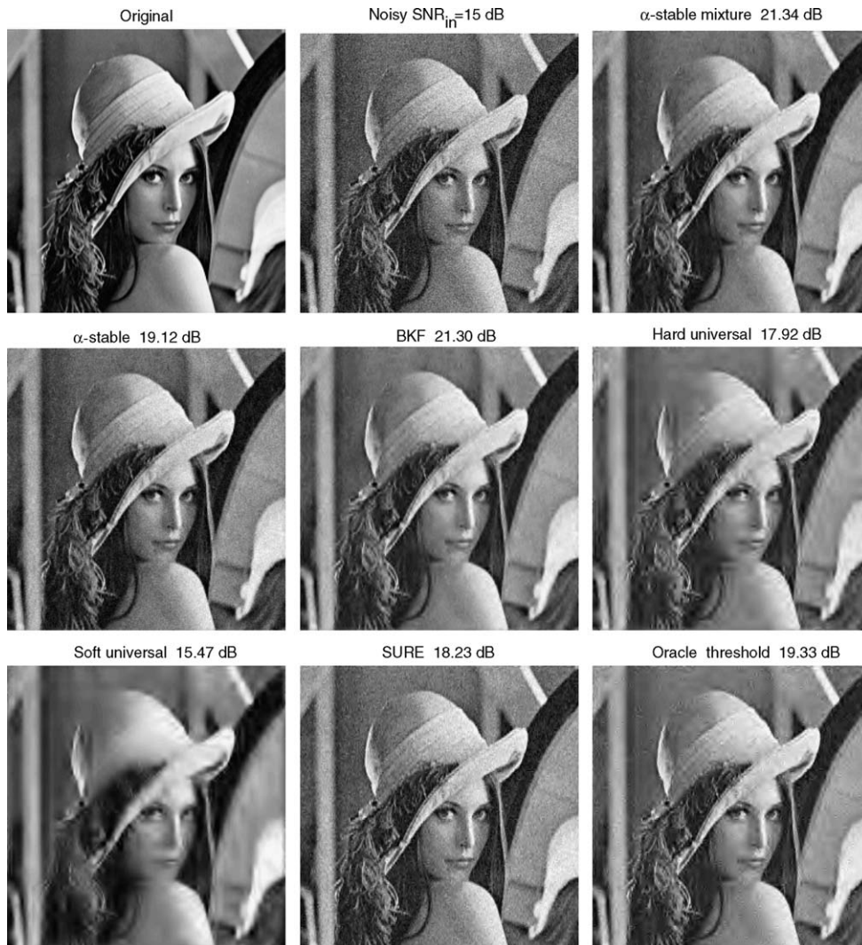
Fig. 5. Visual comparison of various denoising methods on test image Lena. This image is corrupted by Gaussian noise with an input SNR_{in} = 15 dB.
