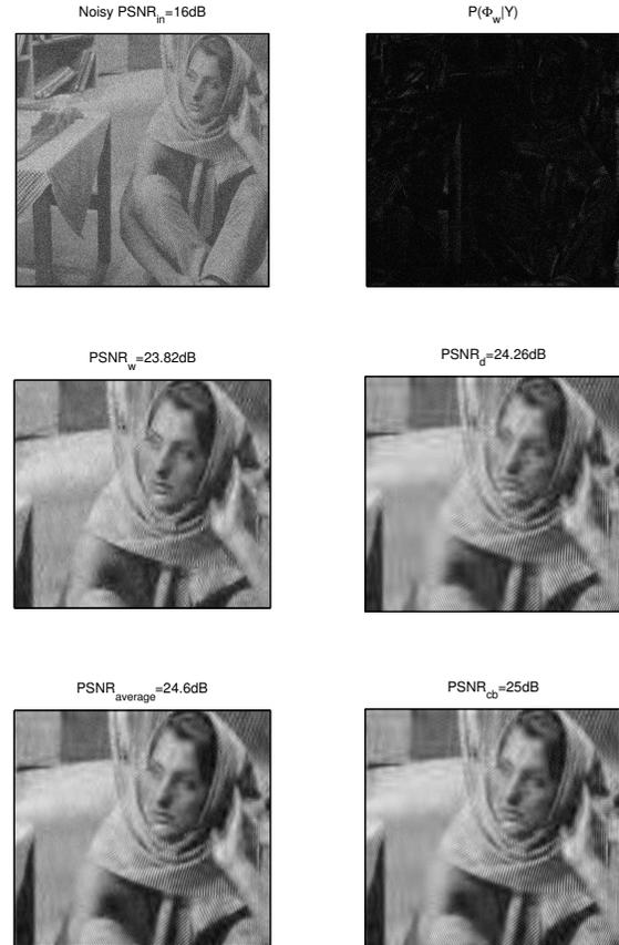
**Fig. 3.** Illustration on the Barbara image with  $\text{PSNR}_{in} = 16\text{dB}$  ( $\sigma_\varepsilon = 40$ ). From top to bottom and left to right: noisy, "wavelet" probability map, estimate in wavelets, estimate in local DCT, combined by averaging, optimally combined estimate.
