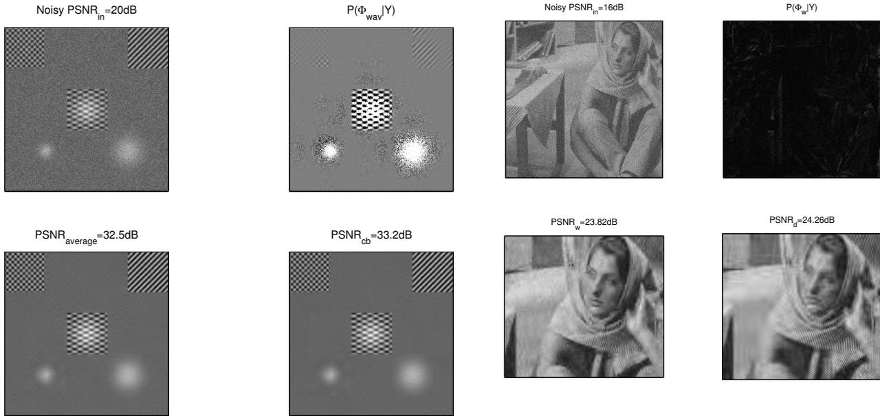
**Fig. 2.** Illustration on a synthetic example (texture+gaussian image with  $\text{PSNR}_{in} = 20\text{dB}$ ). From top to bottom and left to right: noisy, posterior probability map of the wavelet transform, combined estimate by averaging, optimally combined estimate.
