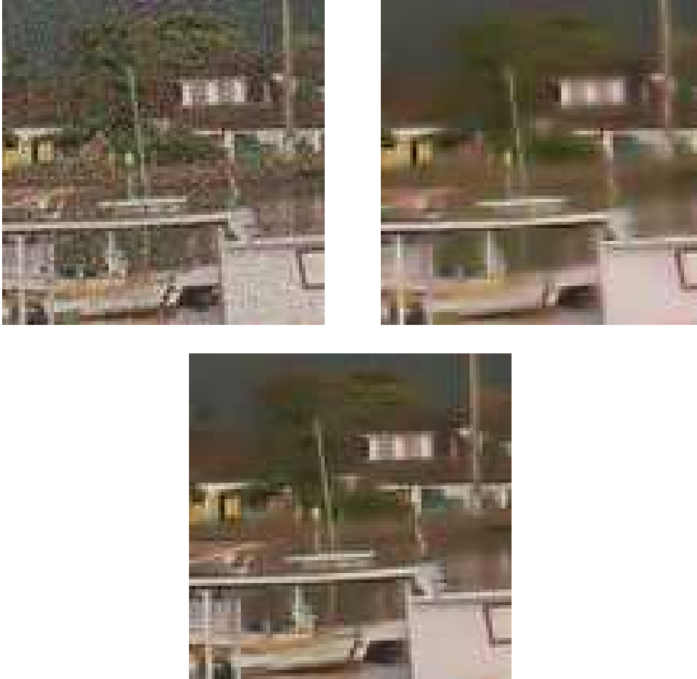
Fig. 24. Zoom the test images. Top-Left : Original image with additive Gaussian noise. The SNR is equal to 15 dB. Top-Right : Wavelet-based denoising in the RGB space. Bottom : Wavelet-based denoising in the curvelet-GMCA space.
