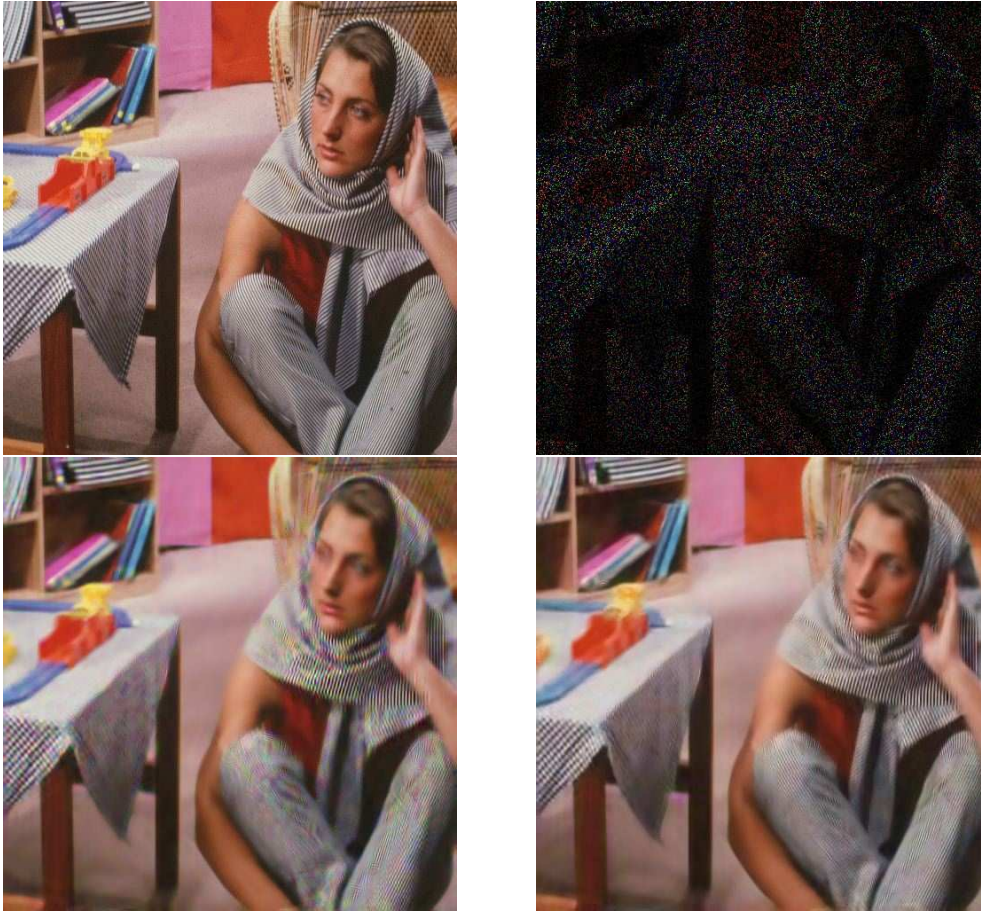
Fig. 26. Recovering color images. (a) Original Barbara color image. (b) Masked image - 90% of the color pixels are missing. (c) Inpainted image using the original MCA algorithm on each color channel. (d) Inpainted image using the adaptive GMCA algorithm.
