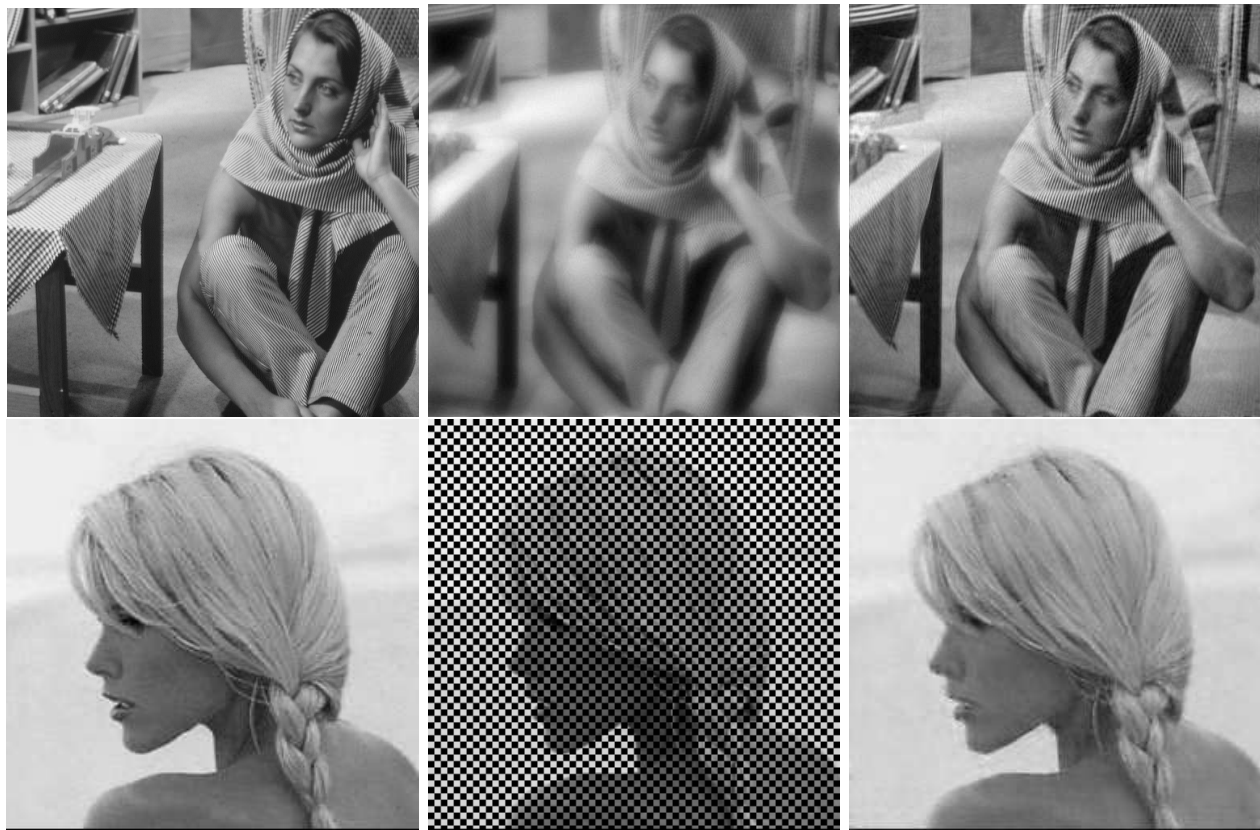
Figure 17: Illustration of the use of curvelets (DCTG2 transform) when solving two typical linear inverse problems: deconvolution (first row), and inpainting (second row). First row: deconvolution of Barbara image, original (left), blurred and noisy (middle), restored (right). Second row: inpainting of Claudia image, original (left), masked image (middle), inpainted (right).
