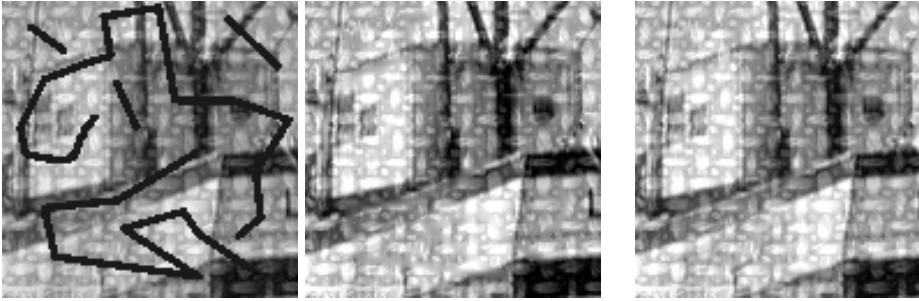
Input Image MCA, SNR=24.9dB Adaptive MCA, SNR=28.6dB FIG. 5.8. Image inpainting with a structured mask containing moderately large gaps.
